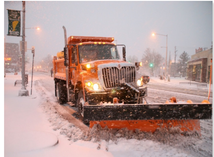
6-wheel Plow Truck with salt dispenser on the back
